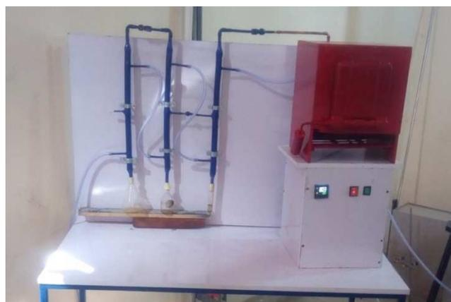
Figure 1. Destructive Distillation Unit for Coal Processing.
