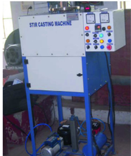
Figure 1. Stir Casting Machine.
